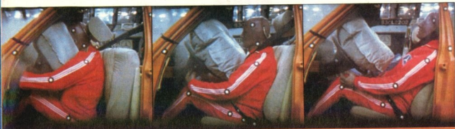
milliseconds it can sense a major frontal impact, inflate the driver's air bag, and tighten the front passenger's three-point seat belt.
